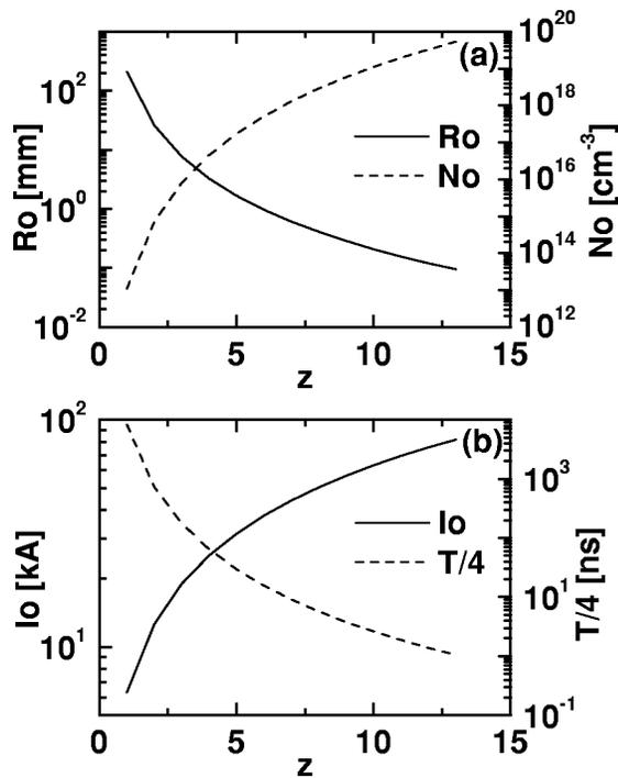
FIG. 4. Experimental parameters suggested by the  $z$ -scaling formulas are plotted with respect to  $z$ : (a) initial radius ( $R_o$ ) and initial density ( $N_o$ ) and (b) peak ( $I_o$ ) of discharge current and its quarter-period ( $\tau/4$ ).
