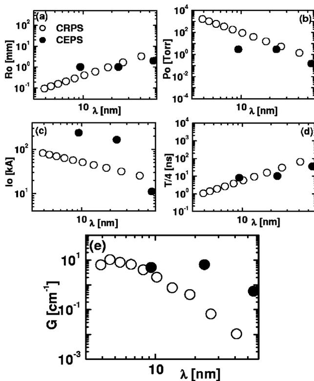
FIG. 5. The suggested experimental conditions for CRPS and CEPS are compared: (a) initial radius ( $R_0$ ), (b) initial density ( $N_0$ ), (c) peak current ( $I_0$ ), (d) quarter-period of current pulse ( $\pi/4$ ), and (e) gain. The data for CEPS have been taken from Ref. 13.
