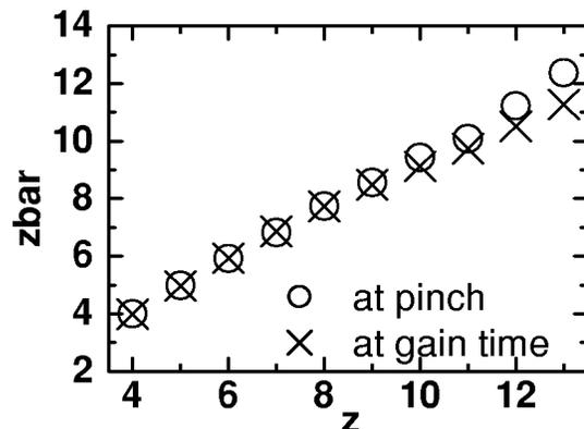
FIG. 3. The average ionic charge,  $\bar{z}$ , at pinch and at the time of maximum gain obtained in the MHD simulation. The good agreement indicates that the assumption of the recombination process being negligible in the early expansion phase, used in the derivation, is valid.
