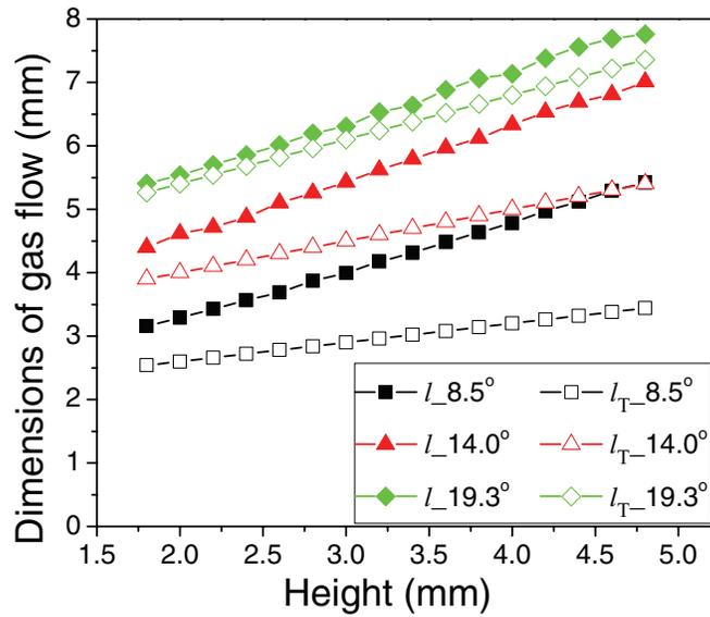
FIG. 5. The comparisons of experimental dimensions (solid symbols) with those predicted by the straight streamline model (open symbols) at different heights for three conical nozzles of  $\alpha = 8.5^\circ$ ,  $14.0^\circ$  and  $19.3^\circ$ .
