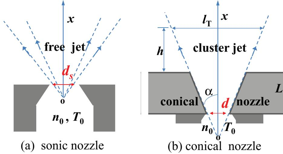
FIG. 1. The schematic diagrams for streamline of gas jet into vacuum from a sonic nozzle (a) and a conical nozzle (b) based on the idealized straight streamline model.
