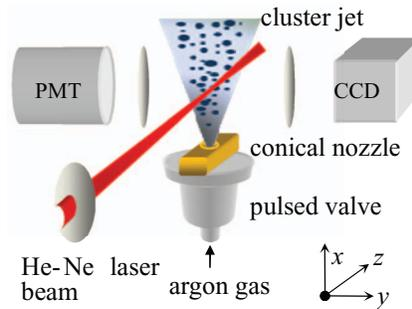
FIG. 2. The schematic diagram of the experimental setup.
