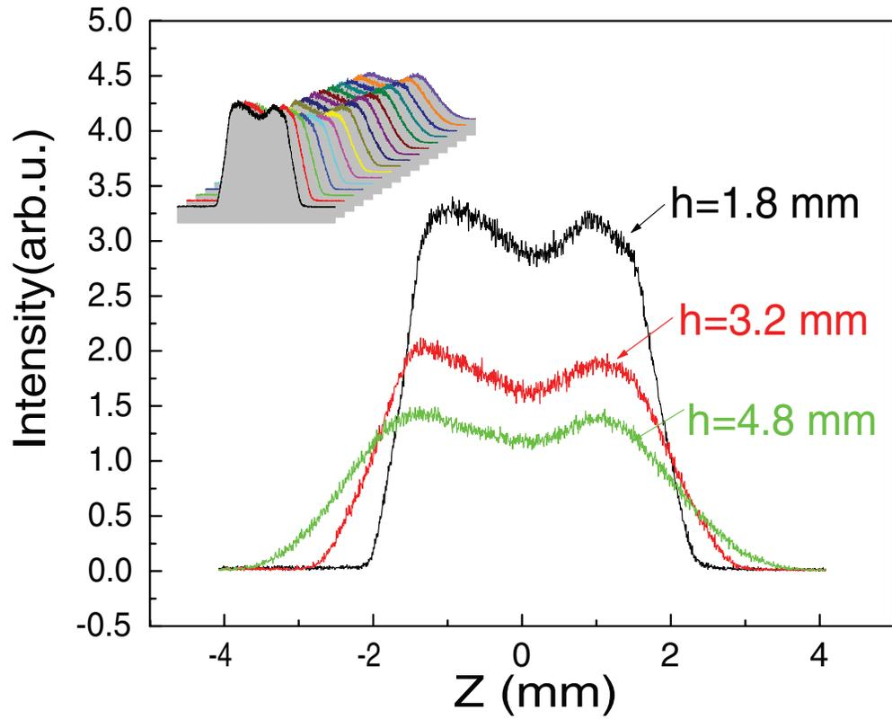
FIG. 4. The profiles of CCD images corresponding to the heights of 1.8 mm, 3.2 mm and 4.8 mm for the conical nozzle of  $\alpha = 14.0^\circ$ . The profiles at all heights were inserted in the top left corner.
