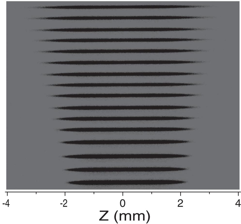
FIG. 3. CCD images at different heights for the conical nozzle of  $\alpha = 14.0^\circ$ . The images from top to bottom correspond to the heights above nozzle which are 4.8 mm to 1.8 mm by a step of 0.2 mm. The laser beam propagates from left to right.
