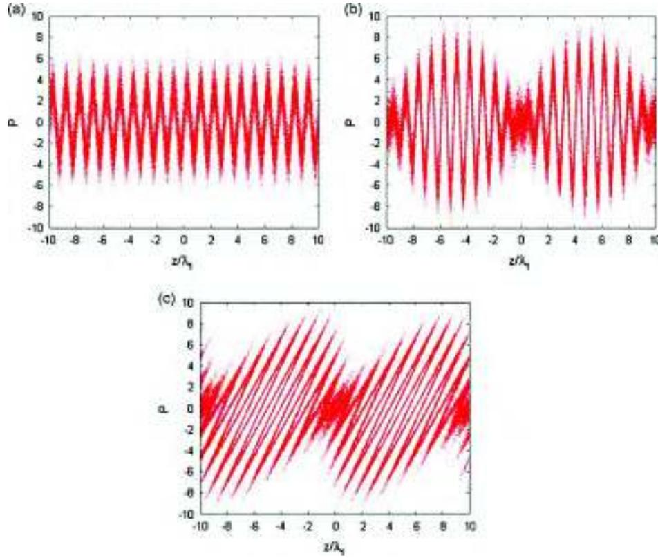
**Fig. 2.** Behavior of the longitudinal phase space distribution of electron beam, (a) after first modulator, (b) after second modulator and (c) after a dispersion section with finite  $R_{56}$ .
