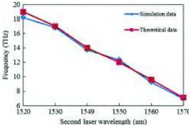
Fig. 7. Tunable THz radiation generation as a function of second laser wavelength. Other parameters are the same as in Fig. 4.
