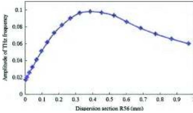
Fig. 6. The amplitude of the THz radiation as a function of  $R_{56}$  (by varying bending angle  $\theta_B$ ). Other parameters are the same as in Fig. 4.
