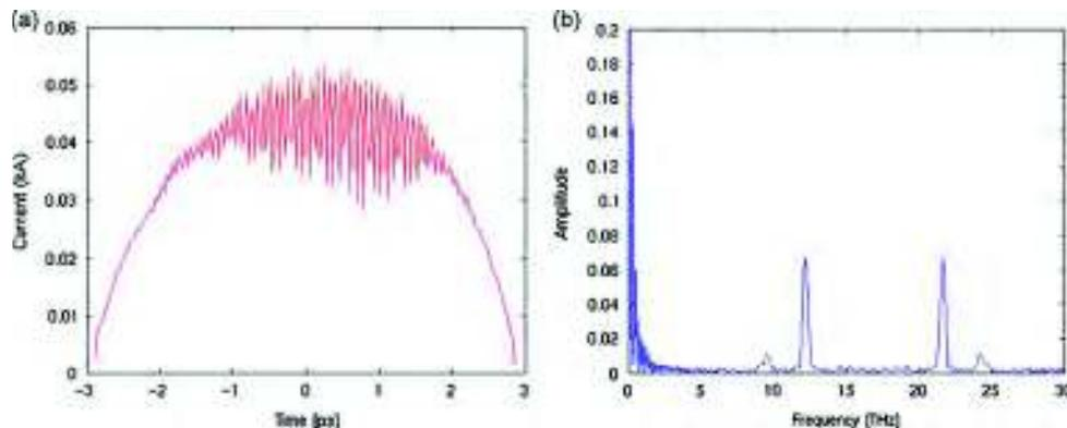
**Fig. 4.** (a) The current modulation of the electron bunch taken after chicane and (b) corresponding FFT spectrum.
