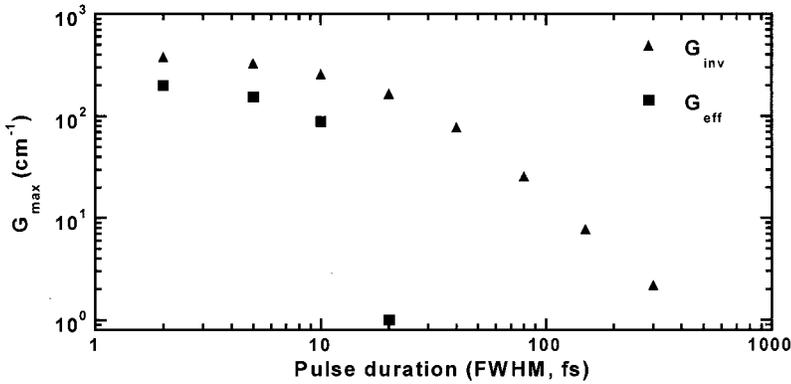
FIG. 4. Change of gain with respect to the pulse duration of pumping x-ray flux of  $10^{20}$  photons/cm<sup>2</sup>. The initial Ca density is  $5 \times 10^{20}$  cm<sup>-3</sup>.
