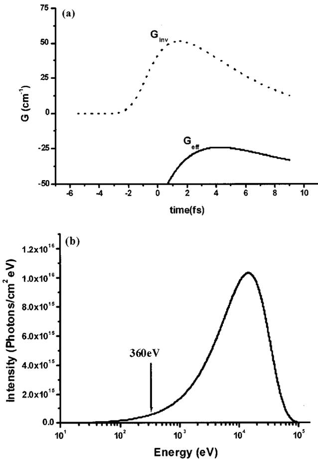
FIG. 5. (a) Temporal change of  $G_{inv}$  and  $G_{eff}$  for the black-body radiation with a temperature of 9 keV and a duration of 5 fs FWHM. (b) The energy distribution of the black-body radiation used in (a). The photon energy of 360 eV indicated by the arrow is slightly above the  $L_{23}$  absorption edge of Ca.
