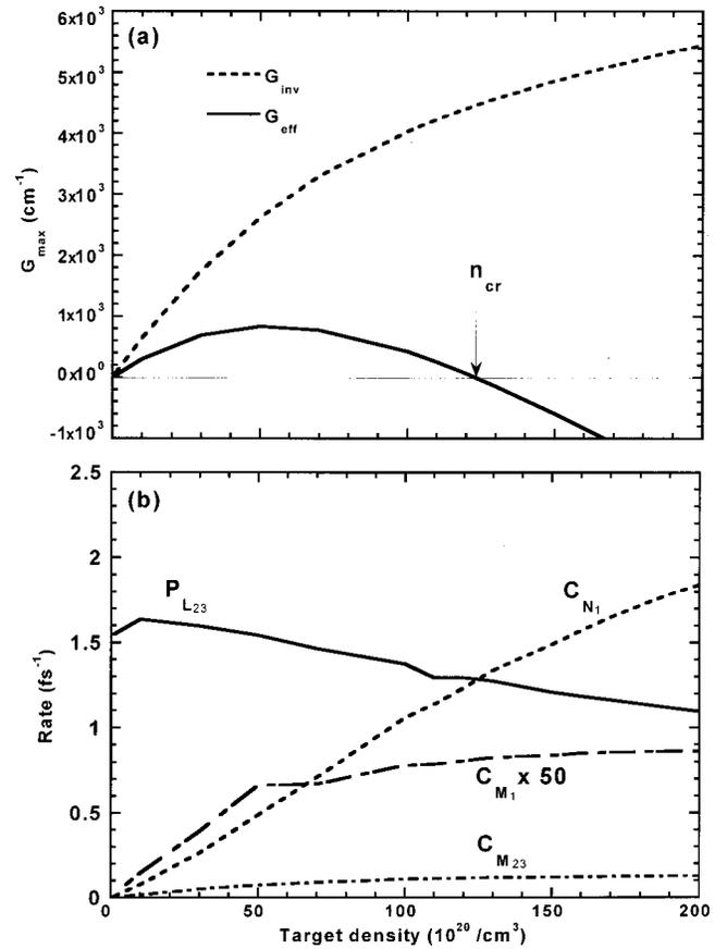
FIG. 3. (a) Behavior of the maxima of  $G_{\text{inv}}$  and  $G_{\text{eff}}$  with respect to the initial Ca density for a given radiation flux of  $1 \times 10^{18}$  photons/cm<sup>2</sup> and a duration of 2 fs FWHM. (b) Behavior of photoionization rates for the  $L_{23}$  IVL ( $P_{L_{23}}$ ), collisional ionization rates for the  $M_1$ , and  $M_{23}$ , IVLs ( $C_{M_1}$ ,  $C_{M_{23}}$ ) at the time of the gain maximum for the same pumping flux as in (a).
