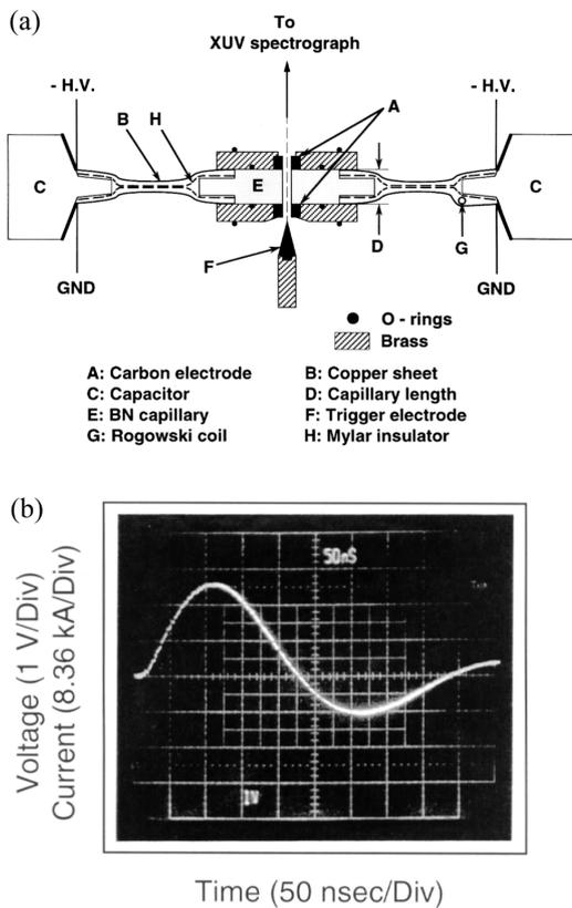
Fig. 1. (a) A schematic diagram of the capillary discharge system. (b) An oscillogram of the current waveform from a 14-mm-long capillary discharge for an input energy density of  $2 \text{ kJ/cm}^3$  at charging voltage of 25 kV.
