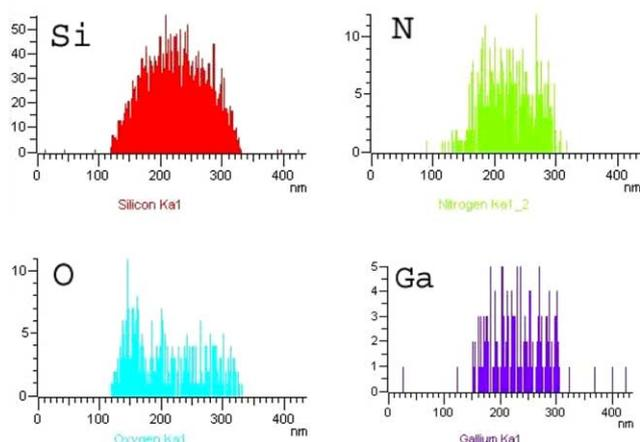
Fig. 4. The line-scan EDX analyses of a nanocable.
