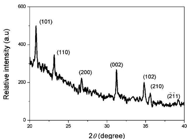
Fig. 2. XRD pattern of the as-prepared sample grown on a Si substrate with GaN.
