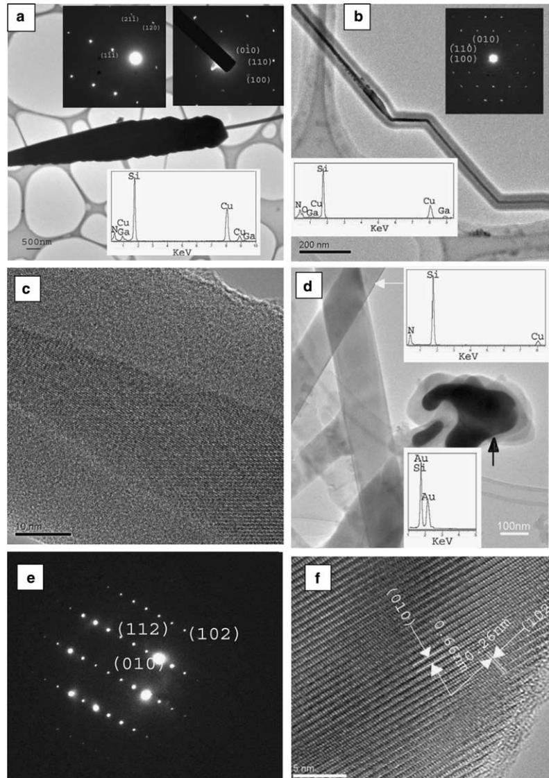
Fig. 3. (a) TEM image of a nanowire with a spearlike tip grown on a Si substrate with GaN. The lower inset is its EDX, and the left upper inset the SAED of the spearlike tip, and the right upper inset SAED of the nanowire. (b) TEM image of a nanocable, upper inset is its SAED, and lower inset is its EDX. (c) A high-resolution TEM image of the nanocable in (b). (d)–(f) are TEM, SAED and HRTEM of the nanowires grown on an Au-coated Si substrate without GaN, respectively.
