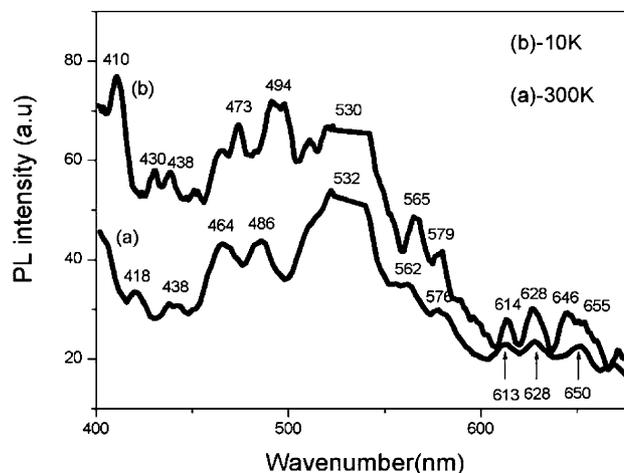
Fig. 5. Photoluminescence of Ga doped  $\alpha$ - $\text{Si}_3\text{N}_4$  based nanowires.
