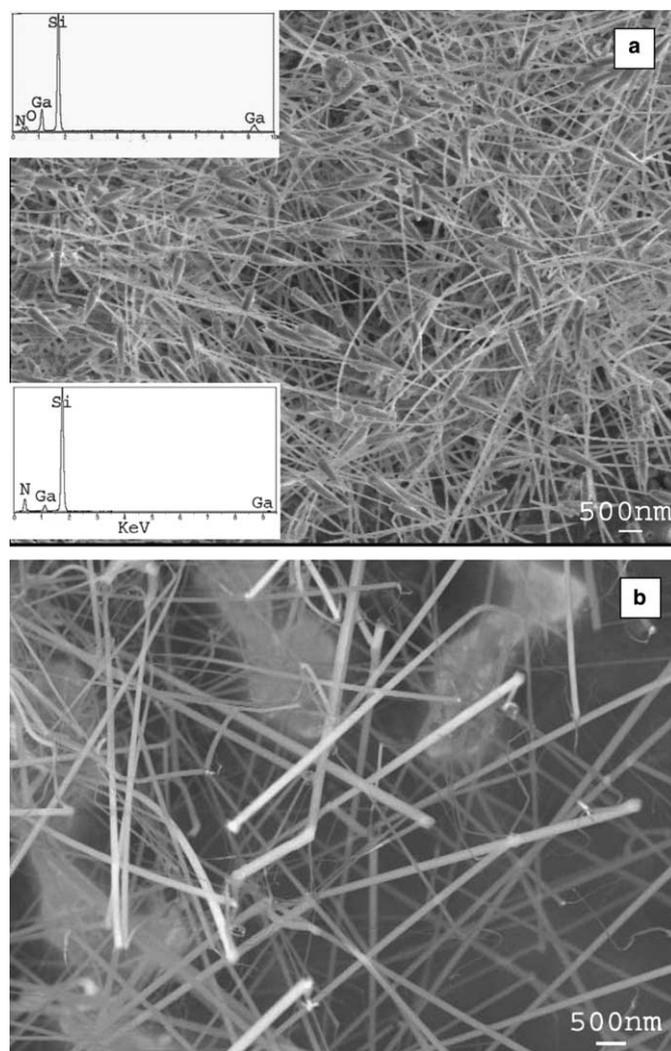
Fig. 1. (a) SEM image of the samples grown on a silicon substrate with GaN. The insets are EDX. (b) SEM image of as-prepared samples grown on an Au-coated silicon substrate without GaN.
