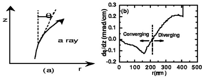
FIG. 4. (a) Schematic drawing of a beam propagation in the  $r$ - $z$  plane; (b) deflected angle per unit length for the case of Fig. 3.
