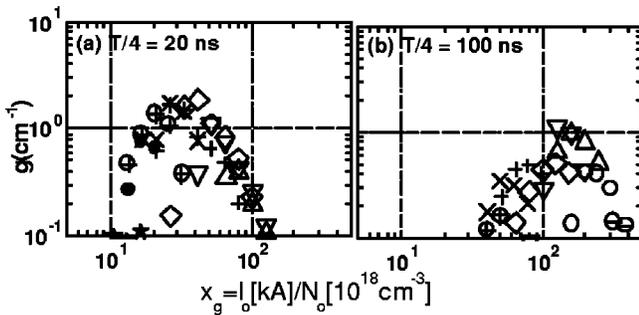
FIG. 1. Gain of C VI  $H_{\alpha}$  (18.2 nm) line is plotted as a function of  $I_o/N_o$  with 30% of theoretical optical trapping for the cases of (a)  $T/4=20$  ns,  $R_o=1$  mm, and (b)  $T/4=100$  ns,  $R_o=2$  mm. The symbols represent initial densities in  $10^{18} \text{ cm}^{-3}$ : ( $\ominus$ ):0.16, ( $\circ$ ):0.25, ( $\triangle$ ):0.40, ( $\nabla$ ):0.63, ( $\diamond$ ):1.0, (+):1.6, ( $\times$ ):2.5, ( $\oplus$ ):4.0, ( $\bullet$ ):6.3, and ( $\star$ ):10.
