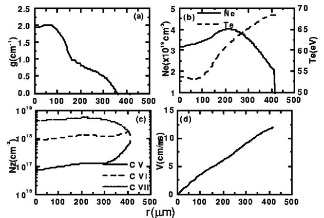
FIG. 3. The radial distributions of plasma quantities at the time of maximum gain, 26.7 ns for the case of Fig. 2: (a) gain of C VI  $H_{\alpha}$  (18.2 nm) line ( $g$ ), (b) the electron density ( $N_e$ ) and the temperature ( $T_e$ ), (c) the population densities of ground states, and (d) the radial velocity.
