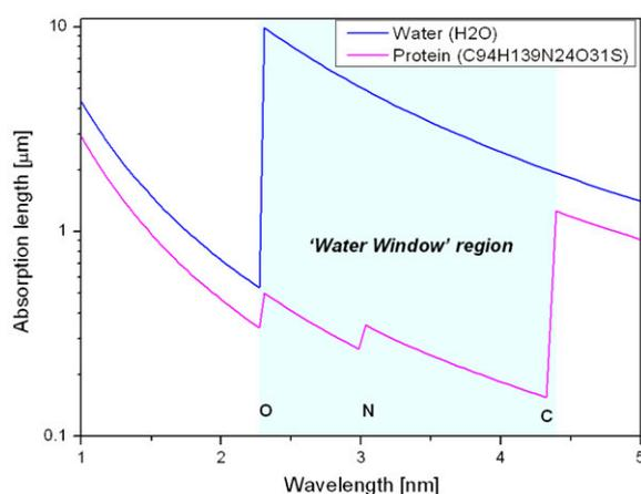
**Figure 1.** The absorption length for soft x-rays in water and protein as a function of wavelength. The spectral range between carbon and oxygen absorption edges is called the 'water window' and offers a natural contrast for biological materials.
