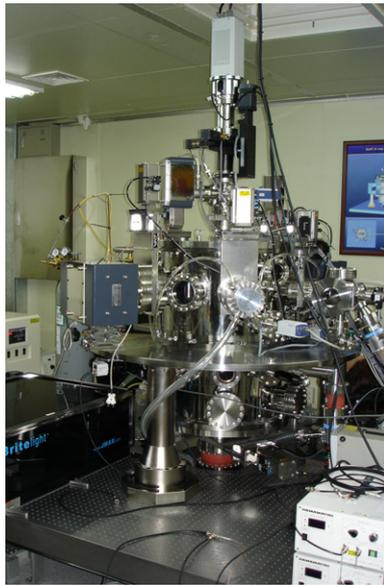
**Figure 5.** Photograph of a vertical type compact soft x-ray transmission microscope system for biomedical application.
