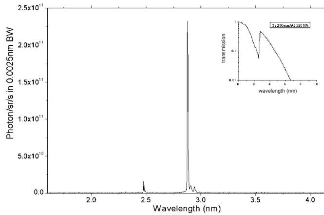
**Figure 3.** Typical spectrum obtained with a Ti/Al filter, showing a quasi-monochromatic source suitable to imaging with zone plates. The spectral resolution at 2.88 nm bandwidth was measured as  $\lambda/\Delta\lambda = 1000$ .
