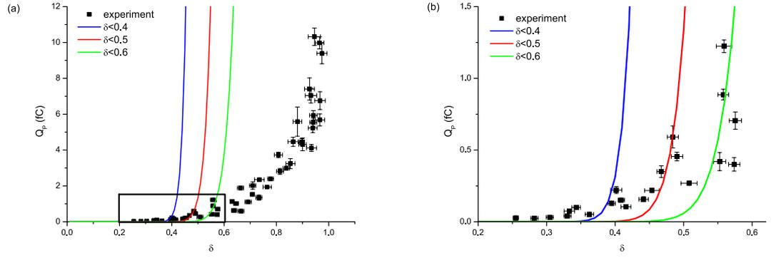
**Figure 4.** (a) Fitted curves by Zener’s formula for transition probability multiplied by a constant which ensures least discrepancy to the experimental data for  $\delta$  smaller than a value given in the legend for calcium fluoride (b) magnified view for black rectangle in the left panel.
