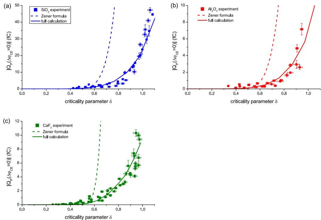
**Figure 3.** Measured maximum transferred charge  $|Q_p(\Delta\varphi_{CE} = 0)|$  as a function of  $\delta$  (squares); fitting based on Zener-Keldysh interband tunneling formula (dashed) and theoretical computations (described in the text) including both interband and intraband transition (solid) for (a) quartz, (b) sapphire and (c) calcium fluoride. Error bars represent the same information as described in the caption of Fig. 2b.
