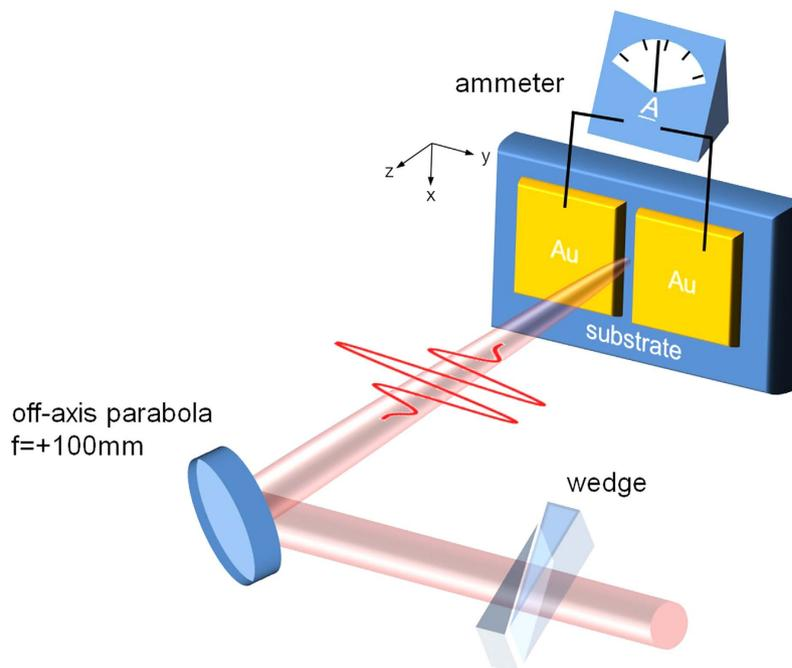
**Figure 1. Schematic of experimental setup.** CEP-stabilized few-cycle optical pulses, polarized perpendicular to the channel between the two gold electrodes, are focused onto the sample by an off-axis parabola. A wedge pair is inserted so that the optical field waveform can be adjusted by introducing an additional CEP.
