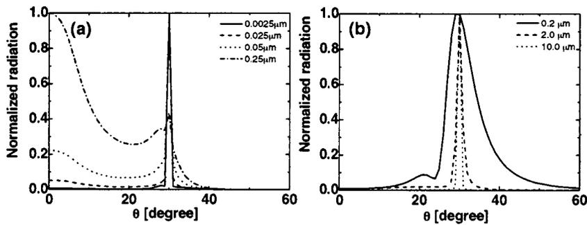
FIG. 8. The dependence of the angular distributions on (a) target thickness and (b) target length is plotted for an electron density of  $10^{15} \text{ cm}^{-3}$ , a width of  $5 \mu\text{m}$ , and  $\xi=15^\circ$ . The length for (a) is fixed at  $10 \mu\text{m}$  and the thickness for (b) at  $2.5 \text{ nm}$ .
