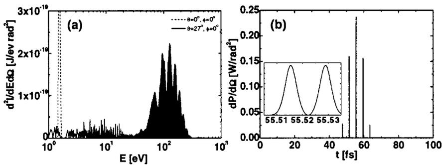
FIG. 2. RNTS by a single electron for a linearly polarized laser pulse of  $4 \times 10^{19}$  W/cm<sup>2</sup> and 20 fs FWHM. (a) Angular harmonic spectrum and (b) angular power at the direction of  $\theta = 27^\circ$  and  $\phi = 0^\circ$ . The inset of (b) shows the enlarged central double peaks. It is shown that the radiation contains energy spectrum from a few tens to 200 eV with a pulse width of 5 fs FWHM.
