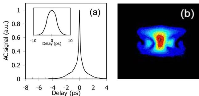
Fig. 3. (Color online) (a) Intensity autocorrelation trace after the compression. Inset, autocorrelation trace of chirped output pulses (b) FROG trace after the compression.
