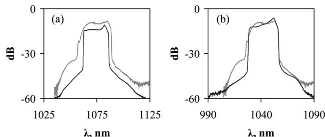
Fig. 2. (a) Spectrum of 9 nJ (black) and 25 nJ pulses (gray) from grating-compensated oscillator. (b) Spectrum of 25 nJ pulses from grating-less compensator (black) and grating-compensated oscillator. The latter is the same data as in (a), scaled to the center wavelength of the grating-less oscillator.
