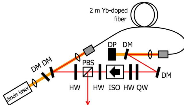
Fig. 1. (Color online) Schematic diagram of a grating-less fiber oscillator: HW, half-wave plate; QW, quarter-wave plate; ISO, isolator; PBS, polarizing beam splitter; DP, beam dumper; DM, dichroic mirror.
