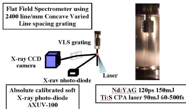
FIG. 1. Experimental setup for water-window source using a liquid nitrogen jet target.
