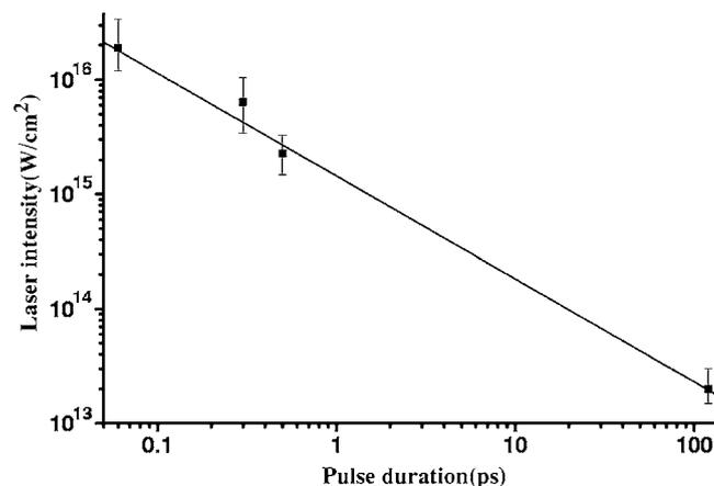
FIG. 6. The laser intensity of the maximum conversion efficiency vs the pulse duration. The data fitting shows that the laser intensity for the maximum conversion efficiency is proportional to  $1/\tau^\alpha$ , where  $\alpha = 0.9 \pm 0.15$ .
