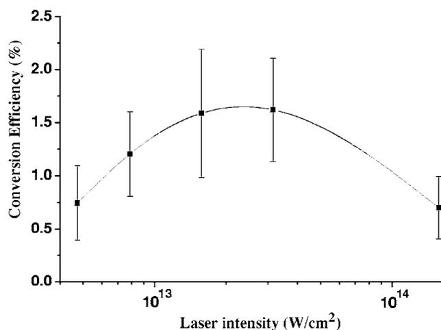
FIG. 4. Conversion efficiency of 532 nm, 120 ps laser light to the 2.88 nm radiation for different laser intensities. The data are connected by a line for the better visibility.
