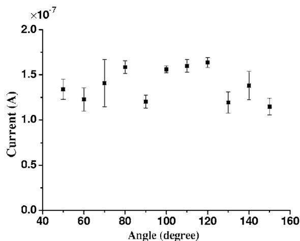
FIG. 3. Angular distribution of the 2.88 nm radiation at a laser intensity of  $1.5 \times 10^{14}$  W/cm<sup>2</sup> of 120 ps pulsed Nd:YAG laser.
