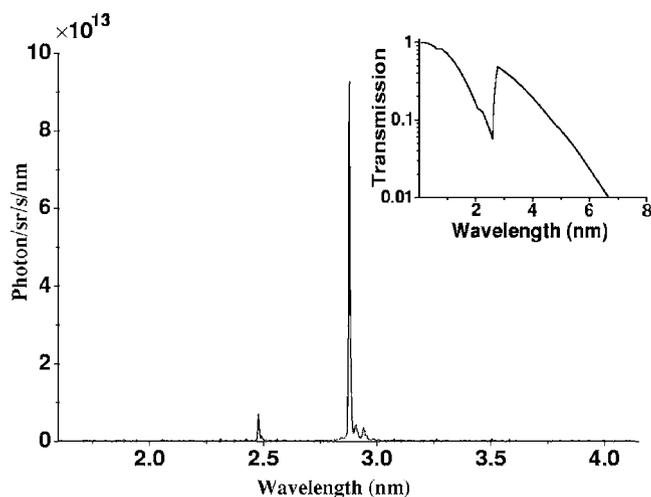
FIG. 2. Spectrum in the water-window region produced from liquid nitrogen at a laser intensity of  $1.5 \times 10^{14}$  W/cm<sup>2</sup> of 120 ps pulsed Nd:YAG laser. A Ti 200 nm/Al 150 nm filter was used for quasimonochromatic spectrum. The inset is the transmission curve of the filter.
