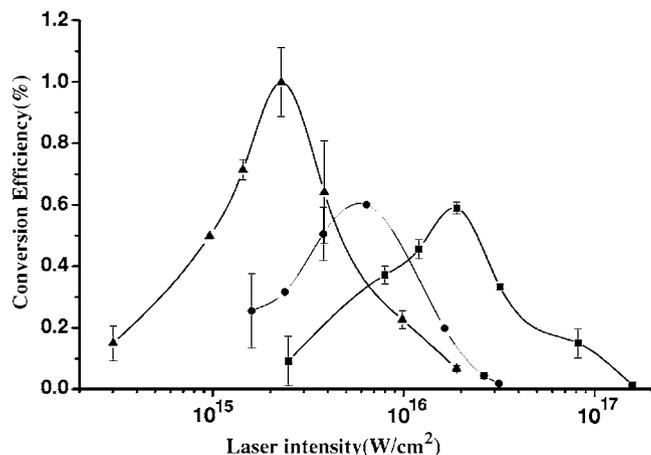
FIG. 5. Conversion efficiency of 800 nm, femtosecond laser light to 2.88 nm radiation (■: 60 fs, ●: 300 fs, and ▲: 500 fs). Data are connected for the better visibility.
