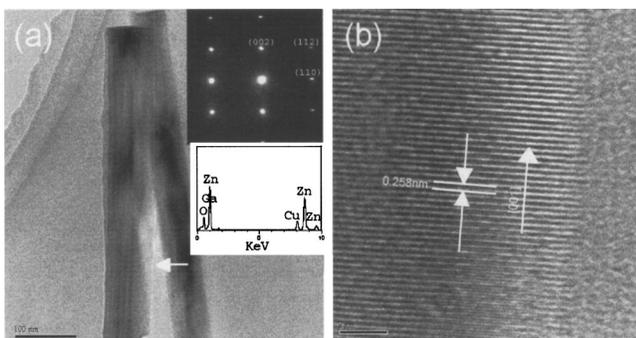
FIG. 3. (a) TEM image of a nanowire grown on the sapphire substrate. The upper inset is SAED; the lower inset is EDX. (b) HRTEM of the corresponding nanowire.
