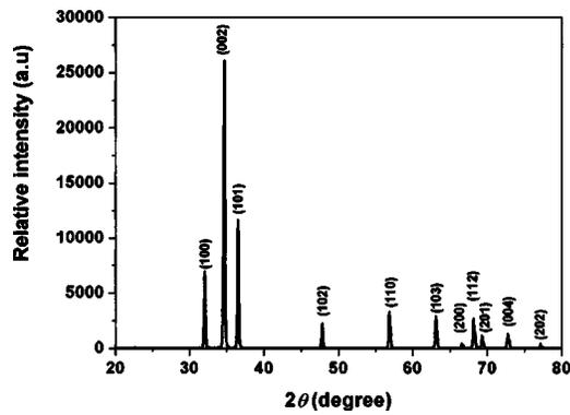
FIG. 2. XRD of Ga-doped ZnO nanowires.
