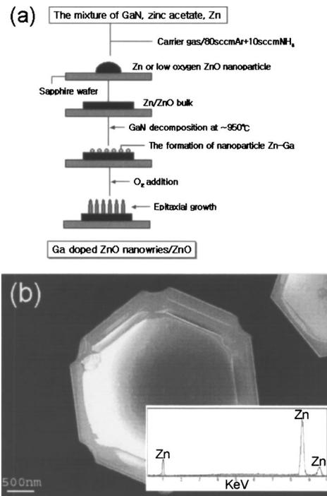
FIG. 5. (a) Formation mechanism of Ga-doped ZnO nanowires. (b) SEM image of a hexagonal Zn particle formed below 700 °C, the inset is for EDX.
