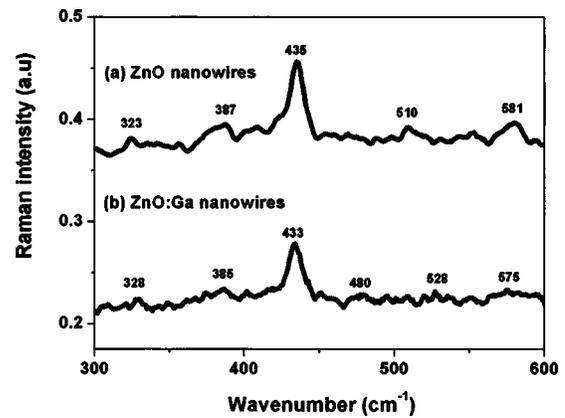
FIG. 4. Raman spectrum of (a) undoped ZnO nanowires grown on a silica substrate and (b) Ga-doped ZnO nanowires/ZnO grown on a sapphire substrate. The excitation was done by 488 nm laser line.
