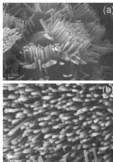
FIG. 1. (a) SEM image of the nanowires grown on a sapphire substrate. (b) Magnified SEM image at a different viewing angle.
