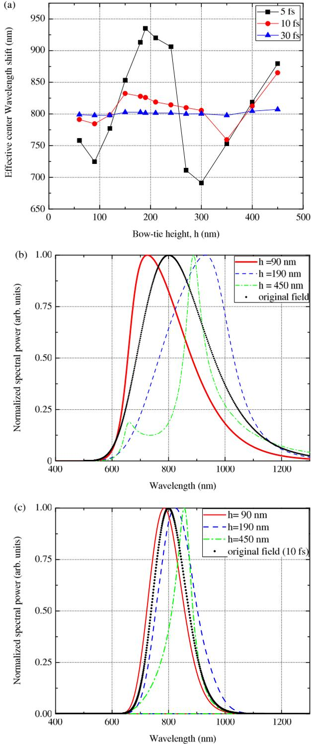
FIG. 3. (a) Effective center wavelength shift for the variation of bow-tie height at three different pulse widths. 5 fs (black squares), 10 fs (red circles), and 30 fs (blue triangles). (b) Resultant spectra of near field for three different bow-tie heights, namely, 90 nm (red solid line), 190 nm (blue dashed line), and 450 nm (green dot-dashed line) for 5 fs pulse excitation. (c) Same as (b), but for 10 fs pulse excitation. In both panels the original field is shown with black circles.
