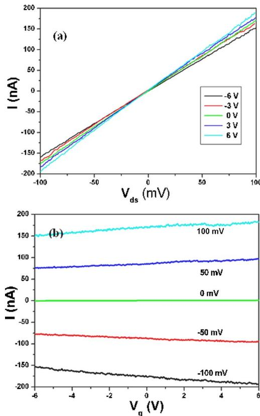
FIG. 2. (Color online) (a) Room-temperature  $I$ - $V_{ds}$  curves at different gate voltages. (b) Transconductance of the Bi-ZnO NW FET under  $V_{ds}=100, 50, 0, -50,$  and  $-100$  mV bias voltages.
