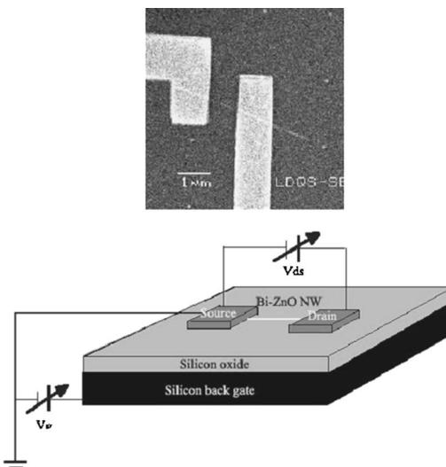
FIG. 1. Scanning electron microscopy image of a Bi-ZnO NW FET with source and drain electrodes.
