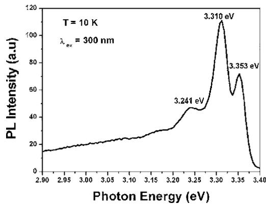
FIG. 3. PL spectra of Bi-ZnO NWs at 10 K excited by 300 nm laser light.
