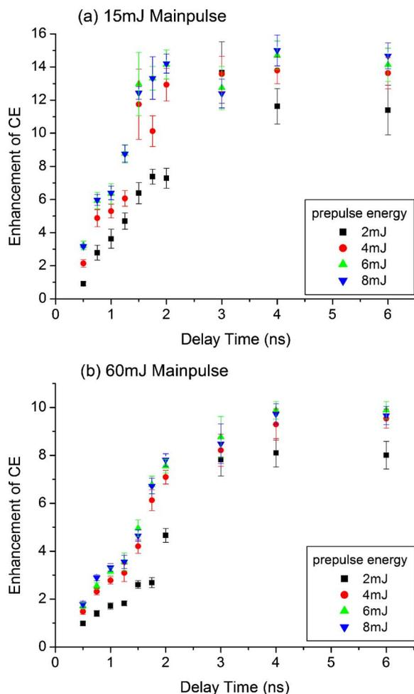
FIG. 4. (Color online) Enhancement of the CE as a function of the prepulse energy and the delay time (a) at 15 mJ main pulse and (b) at 60 mJ main pulse.
