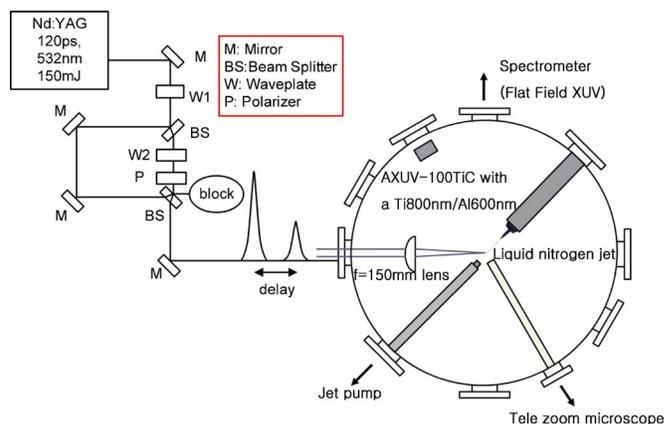
FIG. 1. (Color online) Schematic experimental setup for water-window plasma sources using a liquid nitrogen target. The angle between the jet direction and the laser propagation was 135° due to the experimental arrangement.
