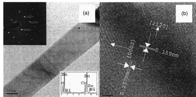
FIG. 3. (a) TEM image of a nanowire. The upper inset is SAED; the lower inset is EDX. Scale bar: 20 nm (b) HRTEM of the corresponding nanowire. Scale bar: 2 nm.
