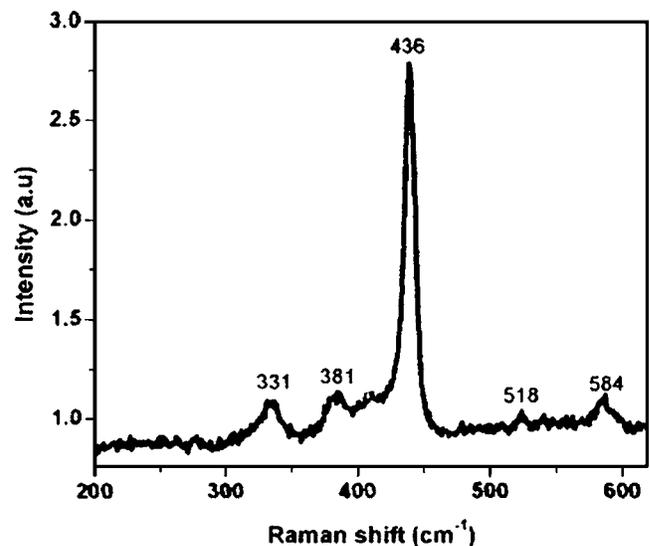
FIG. 4. Raman spectrum of ZnO nanowires grown on an oxidized Si substrate. The excitation was done by a 488-nm laser line.
