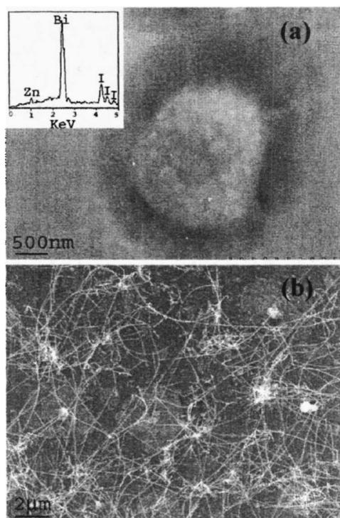
FIG. 5. (a) SEM image of as-prepared samples fabricated without the introduction of oxygen. The inset is for EDX. (b) SEM image of ZnO nanowires around 200 °C.
