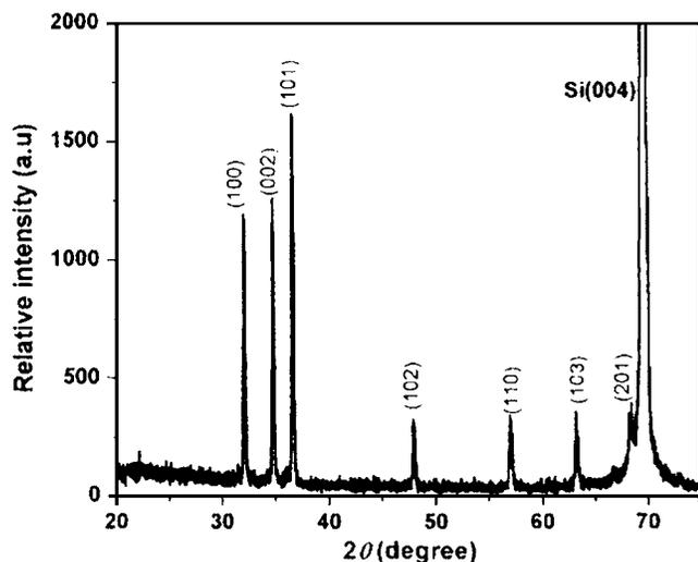
FIG. 2. XRD pattern of ZnO nanowires.
