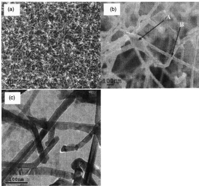
FIG. 1. (a) SEM image of the nanowires grown on an oxidized Si substrate. (b) Magnified SEM image of nanowires with spearlike tips. (c) TEM image.
