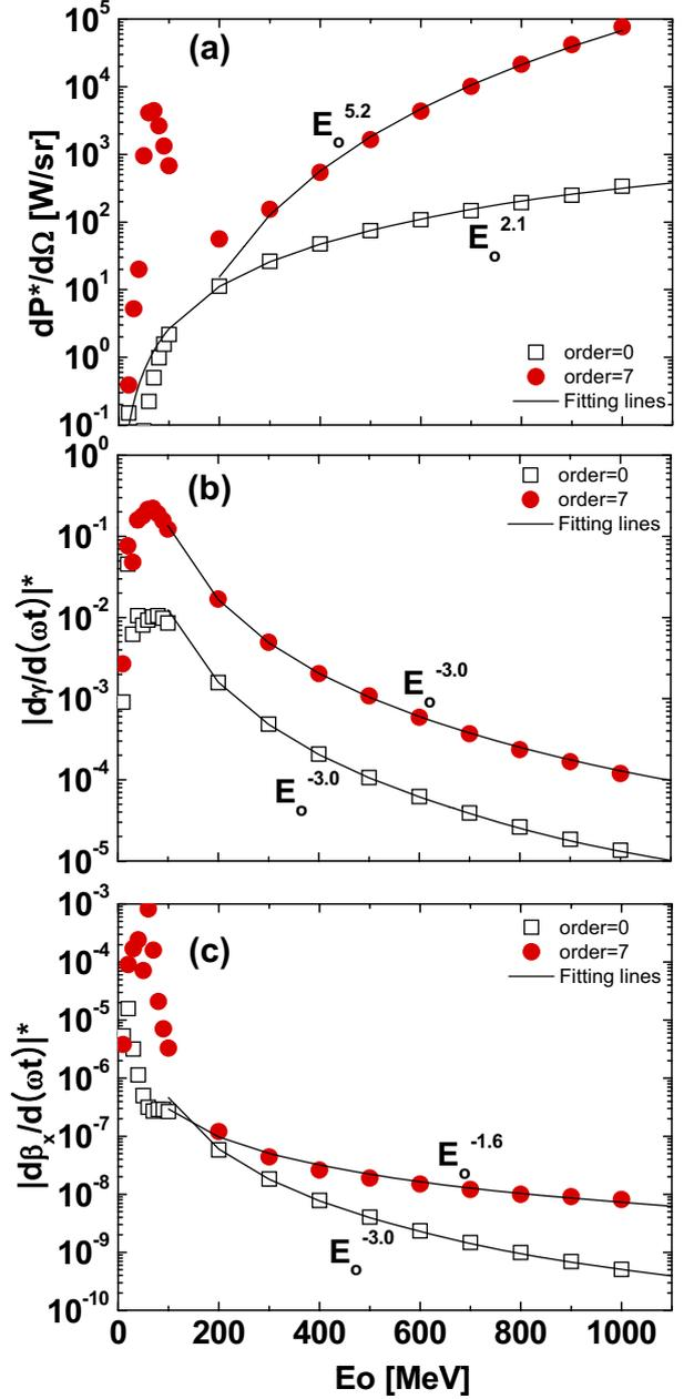
Fig. 8: (Colour on-line) For the co-propagation scheme, the peak values of (a) the angular power in the direction of maximum radiation, (b)  $|\mathrm{d}\gamma/\mathrm{d}\tau|$ , and (c)  $|\mathrm{d}\beta_x/\mathrm{d}\tau|$  vs. the initial electron energy for the paraxial laser beam and the laser beam including fields up to the 7th-order field are compared. For initial energies as high as 200 MeV and above, the scaling laws are obtained by a numerical fitting.
