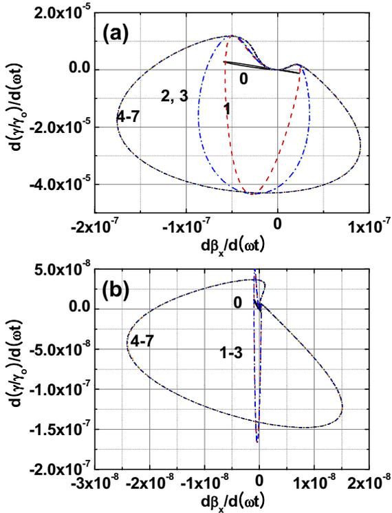
Fig. 4: (Colour on-line) For the co-propagating case, the time derivatives of  $\beta_x$  and  $\gamma/\gamma_0$  are plotted by including the high-order laser fields for (a) 200 MeV and (b) 800 MeV electrons. The laser parameters used are the same as in fig. 3. The numbers on the plots indicate the order up to which the high-order fields are included.
