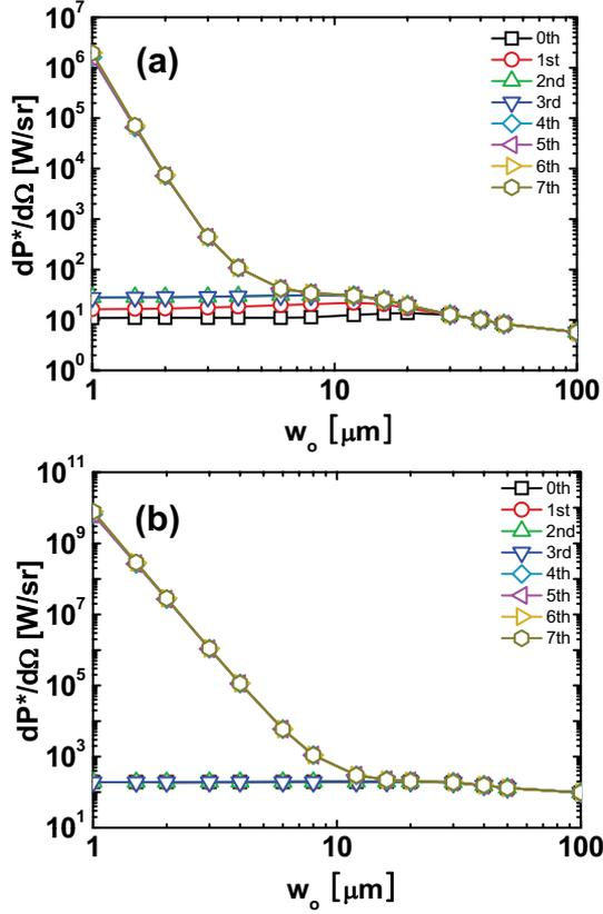
Fig. 7: (Colour on-line) For the co-propagation scheme, the change in the peak angular power with respect to the beam waist size is plotted for (a) 200 MeV and (b) 800 MeV electrons while including the high-order laser fields.
