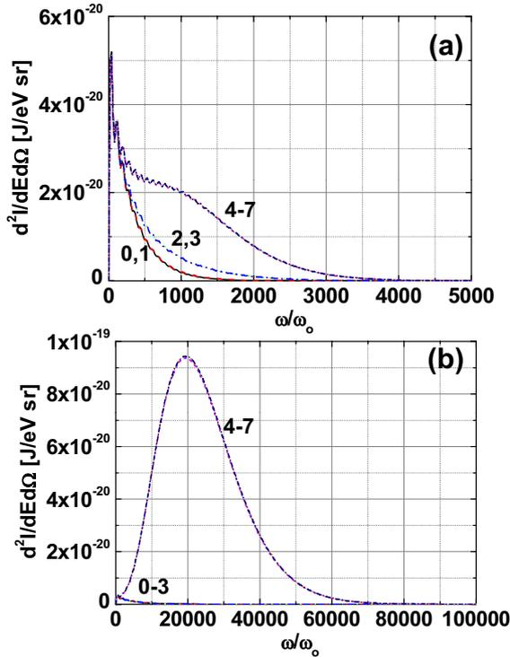
Fig. 5: (Colour on-line) For the dynamics shown in fig. 4, the angular radiation spectra for (a) 200 MeV and (b) 800 MeV are calculated and plotted, including the high-order fields. The spectra were obtained in the direction of maximum radiation, which is the same as that of the laser propagation.
