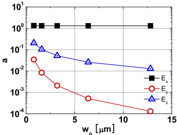
Fig. 1: (Colour on-line) Each component of the laser electric fields is plotted with respect to the beam waist size in units of the normalized vector potential. The laser field is evaluated at  $(w_o/2, w_o/2, 0)$  for a zeroth-order laser intensity  $a_0 = 2.2$ .
