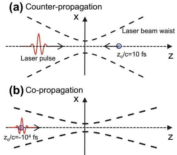
Fig. 2: (Colour on-line) Schematic diagrams for (a) the counter-propagation and (b) the co-propagation interaction scheme between a relativistic electron and a laser pulse.
