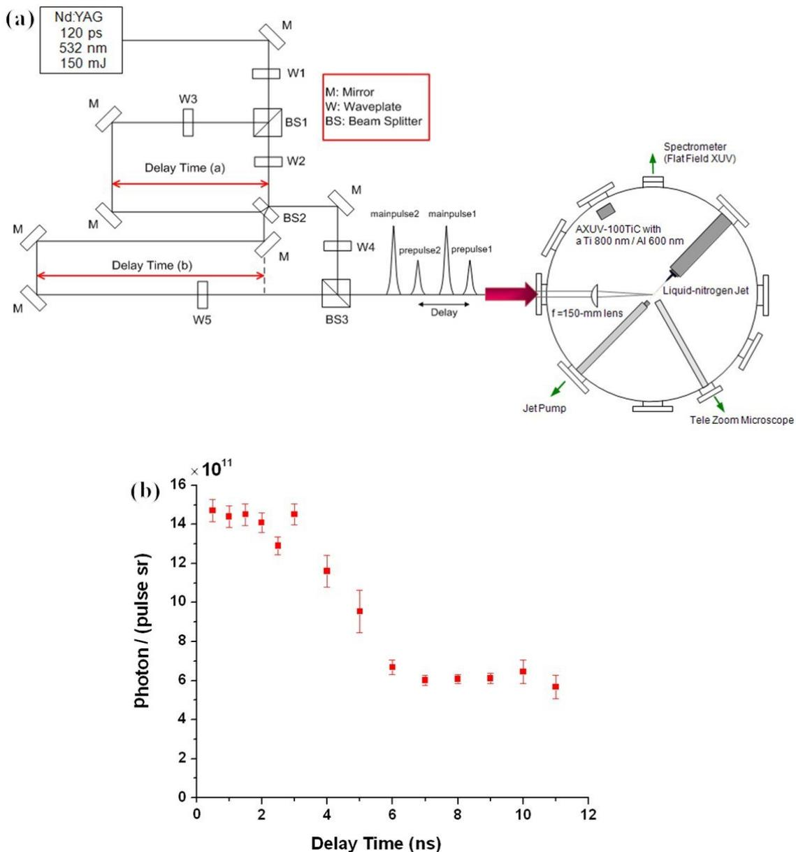
Fig. 4. (a) Schematic experimental setup for the study of the multiple pulse effect. The angle between the jet direction and the laser propagation was  $135^\circ$  due to the experimental arrangement. (b) Photon number as a function of the delay between two pairs of a pre-pulse and a main pulse.
