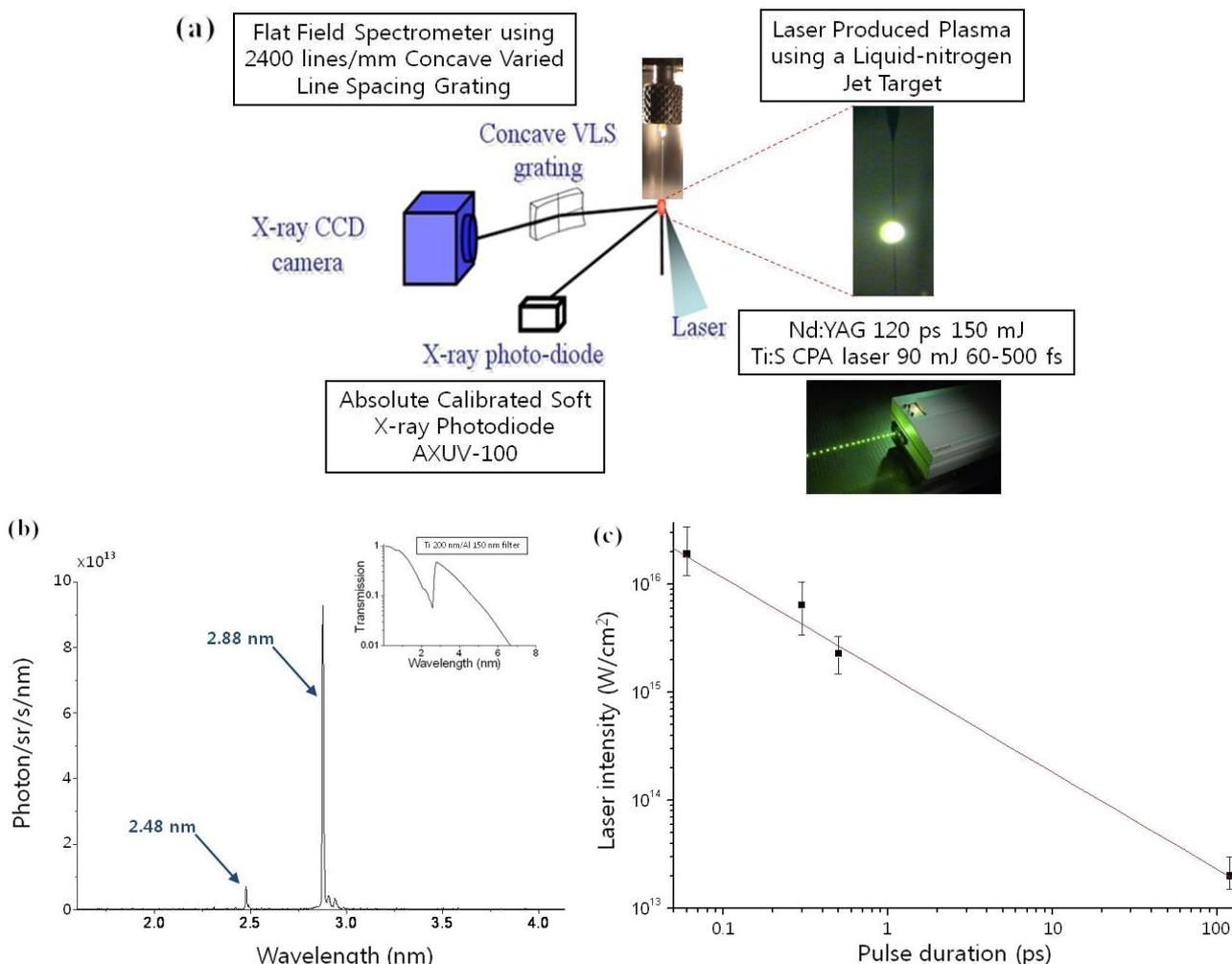
Fig. 1. (a) Experimental setup for a water-window source using a liquid-nitrogen jet target. (b) Spectrum in the water-window region produced from liquid nitrogen at a laser intensity of  $1.5 \times 10^{14}$   $\text{W}/\text{cm}^2$  from a 120-ps pulsed Nd:YAG laser. A Ti 200 nm/Al 150 nm filter was used for the quasi-monochromatic spectrum. The inset is the transmission curve of the filter. (c) The laser intensity of the maximum conversion efficiency vs the pulse duration.
