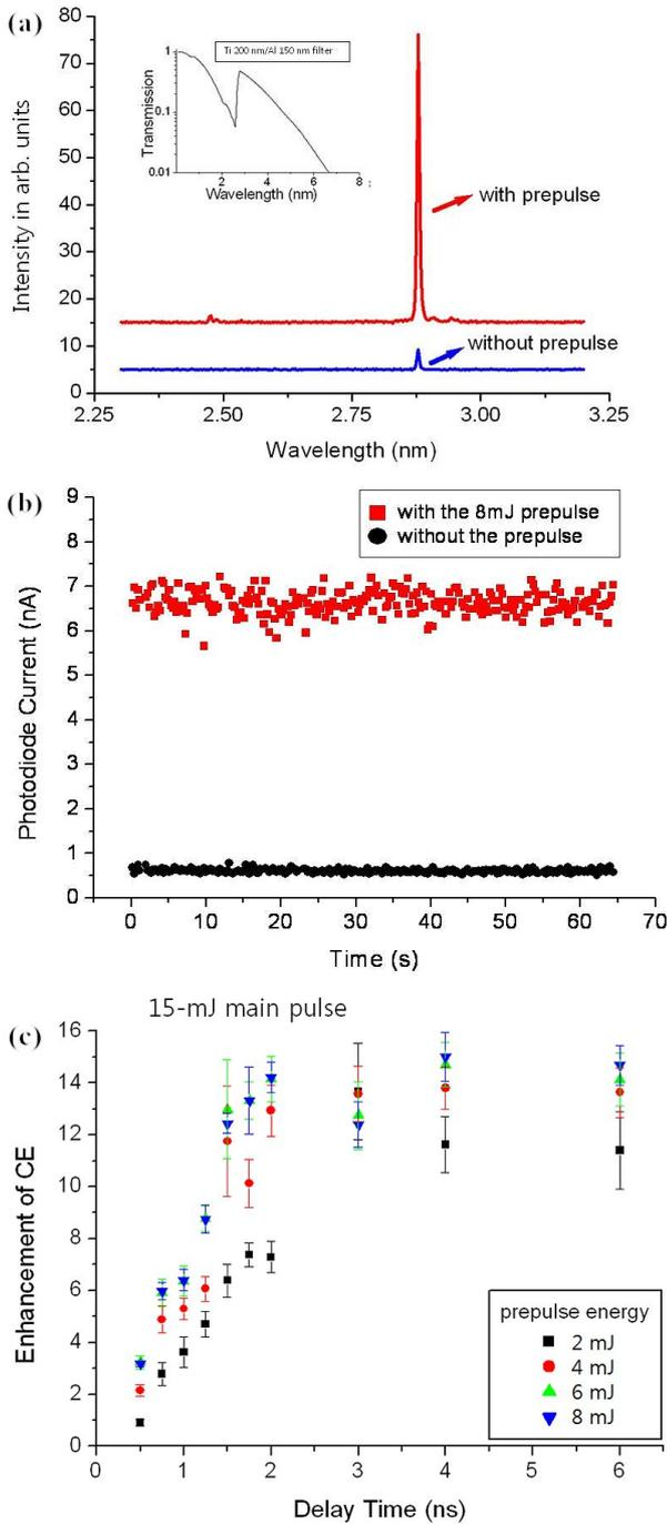
Fig. 3. (a) Spectra and (b) photodiode current with and without the pre-pulse: 60-mJ main pulse, 8-mJ pre-pulse and 6-ns delay. The spectra of the water-window region were obtained with a Ti 200 nm/Al 150 nm filter. The transmission of this filter is shown in the inset of (a). (c) Enhancement of the CE as a function of the pre-pulse energy and the delay time at the 15-mJ main pulse.
