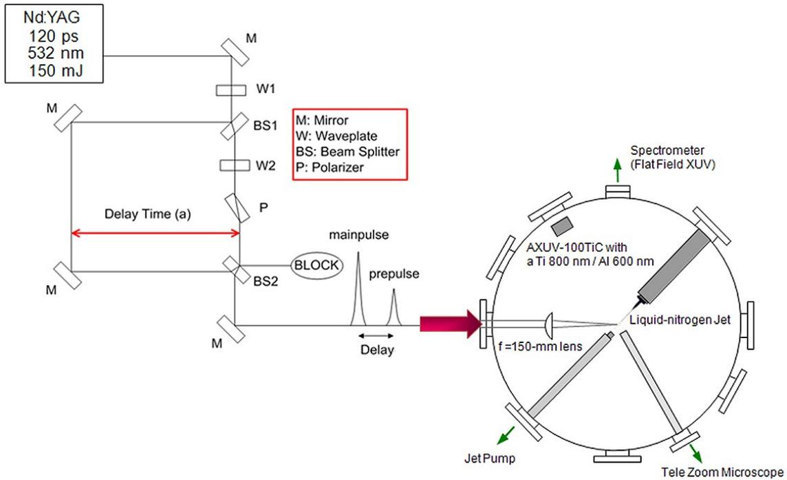
Fig. 2. Schematic experimental setup for the study of the pre-pulse effect. The angle between the jet direction and the laser propagation was  $135^\circ$  due to the experimental arrangement.
