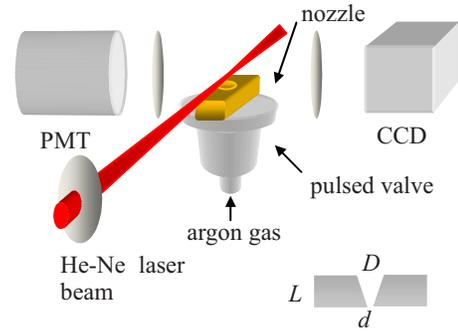
FIG. 1. (Color online) Schematic diagram of the experimental setup. The schematic side cross sectional view of a conical nozzle geometry is shown in the right low corner ( $d=0.5$  mm,  $L=5.0$  mm, and the sonic nozzle is made of stainless steel and the conical nozzles are made of brass).
