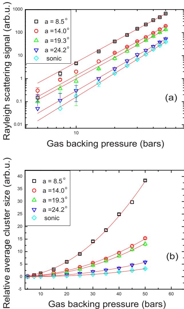
FIG. 2. (Color online) Pressure dependence of (a) Rayleigh scattering signal and (b) the relative average cluster size for different conical nozzles and a sonic nozzle. The solid lines represent the fit to the data.
