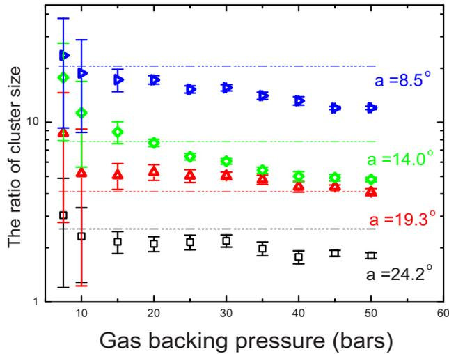
FIG. 4. (Color online) Experimental ratio  $\eta_{\text{exp}}$  of the relative average cluster size for different conical nozzles to that for the sonic nozzle with a 500  $\mu\text{m}$  diameter orifice. The dashed lines represent the ratios  $\eta$  expected by Hagena's scaling law for different conical nozzles. Note that the large errors at lower backing pressure result from the fluctuation of weak Rayleigh scattering signal.
