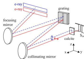
FIG. 6. (Color online) Schematic diagram of the spectrometer with a calcite crystal. The solid line shows the light path for *o* ray whose polarization is horizontal. The dashed line shows the path for *e* ray whose polarization is vertical.
