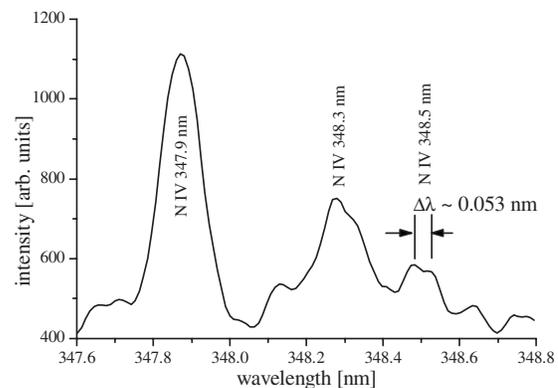
FIG. 10. Measurement of spectral resolution.
