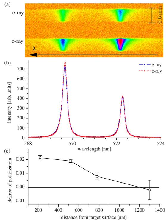
FIG. 9. (Color online) PR spectra. (a) PR spectral image on the focal plane. (b) The cross section of (a) at 200  $\mu\text{m}$  from the target surface. The open circle is *o* ray spectrum and the closed circle is *e* ray. (c) The measured degree of polarization at different distances from the target surface.
