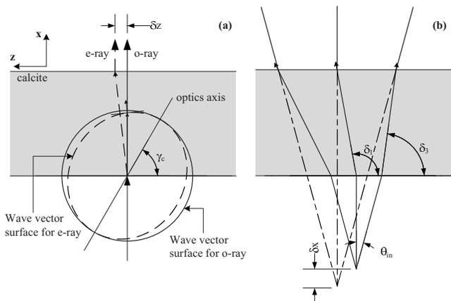
FIG. 5. Ray displacement by a calcite crystal. (a) The displacement of *e* ray. (b) The source displacement.
