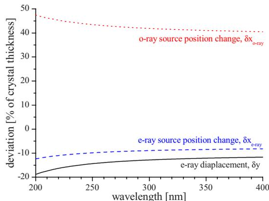
FIG. 7. (Color online) Displacement of the source for different wavelengths at an optic axis of 50°.
