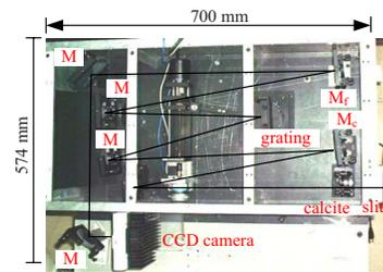
FIG. 3. (Color online) A picture of the spectrometer.  $M_c$  is the collimating mirror and  $M_f$  is the focusing mirror. Flat mirrors are used as folding mirrors to reduce the size of the spectrometer indicated  $M$ .
