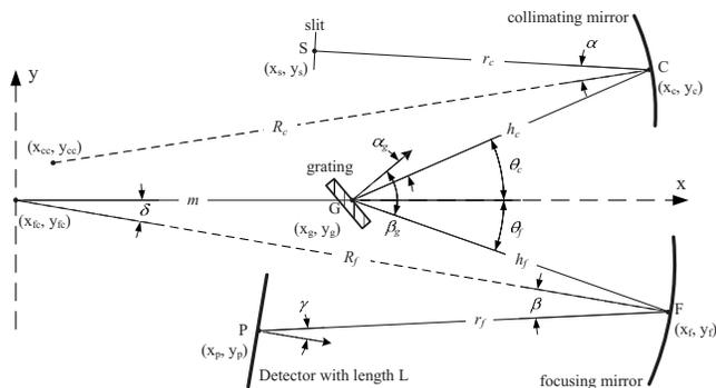
FIG. 1. Schematic diagram of a CTS. *S*, *C*, *G*, *F*, and *P* denote the center of slit, collimating mirror, grating, focusing mirror, and detector, respectively.  $R_c$  and  $R_f$  are the radii of curvature of collimating and focusing mirrors, respectively. Dashed line indicates the normals of the mirrors.
