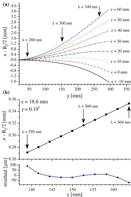
FIG. 2. (Color online) Focal plane position.  $\epsilon$  is the correction factor of the grating position. (a) The focal plane in a wide spectral range with different  $\epsilon$ . (b) The focal plane with flat condition. In (b), dots are the calculated focal position with different wavelengths. The solid line is the linear fit of the focal positions.
