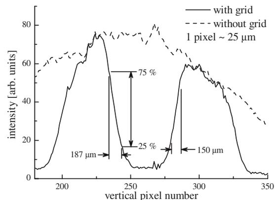
FIG. 4. Measurement of the spatial resolution using a grid at the entrance slit position. The slit was illuminated by a standard lamp.
