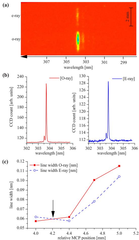
FIG. 8. (Color online) Measured spectrum with Hg standard lamp. (a) The measured spectrum. (b) The cross section of the spectrum. (c) The change of the spectral width of Hg 303.7 nm line for different detector positions.
